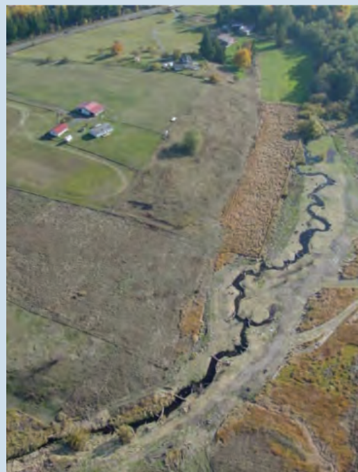
Restoration by remeandering a part of Chimacum Creek
